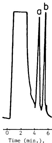
Fig. 2. Chromatogram of cefazolin in muscle tissue of Wistar rat. The tissue extract was treated with methylene chloride. The cefazolin peak (a) had a retention time of 4.65 min. The internal standard (sulfasuxidine) peak (b) had a retention time of 5.87 min.
